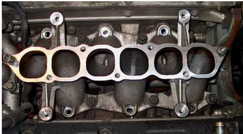
Below is 6G74 3.5L block with smaller 3.0L 6G72 lower intake manifold
