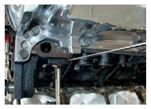
Rear of Engine block partially cut, I had to cut the rest of these 3 bosses off then file it down by hand This really should have been done by a machine shop but I took my time and it is working fine
