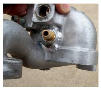
I had to modify the 6G74 main block itself so that the rear engine mount would fit correctly. I have been told that this modification does not have to be done if you use a 94-96 Montero Block. Rear of Engine block before cut
