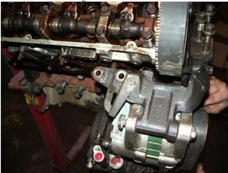
A 6g72 P/S pump bracket and idler pulley is too close to timing belt idler pulley
