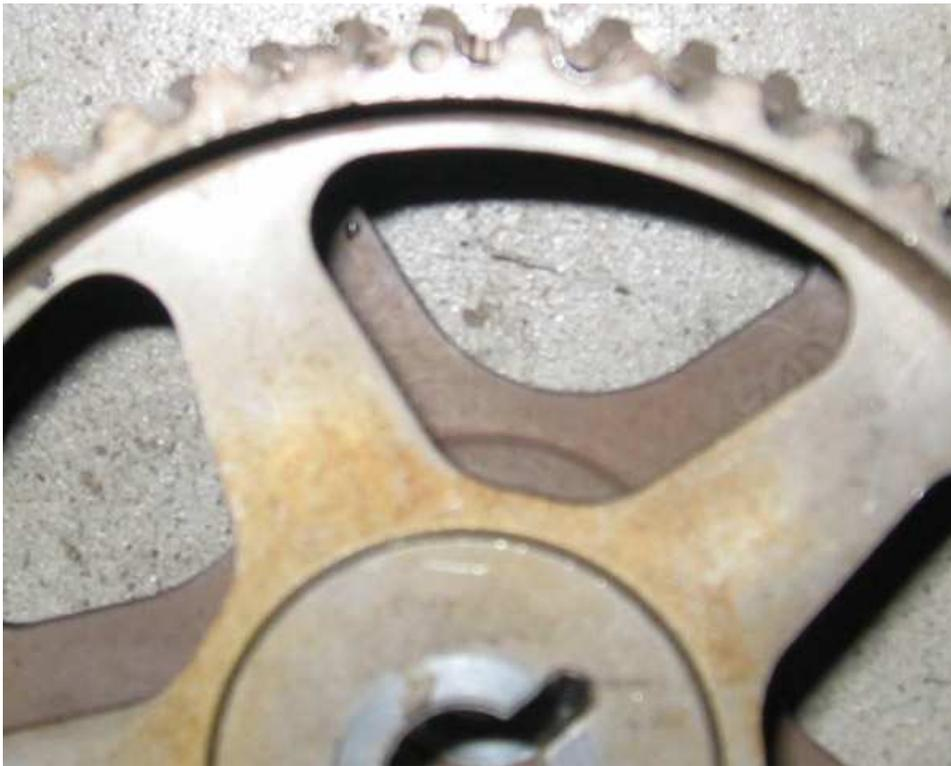
6G74 cam gear has a line between the teeth, this is the one you need.
