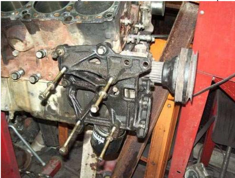
The DOHC Montero harmonic balance will not work in a 3s, next to a Lightweight aluminum 3S crank pulley
