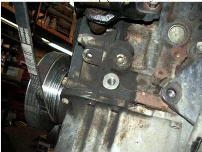
Once the plug is removed the adpater from a 6G72 engine can be installed
