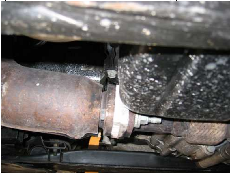
Spacer I added to Exhaust so that I could use stock downpipe.
