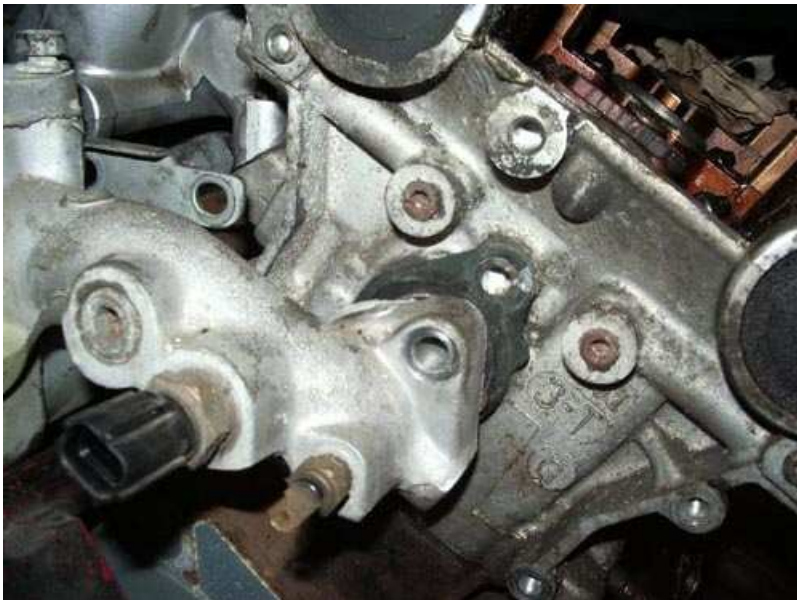
The DOHC Montero Lower intake has rounder holes but it will still work
