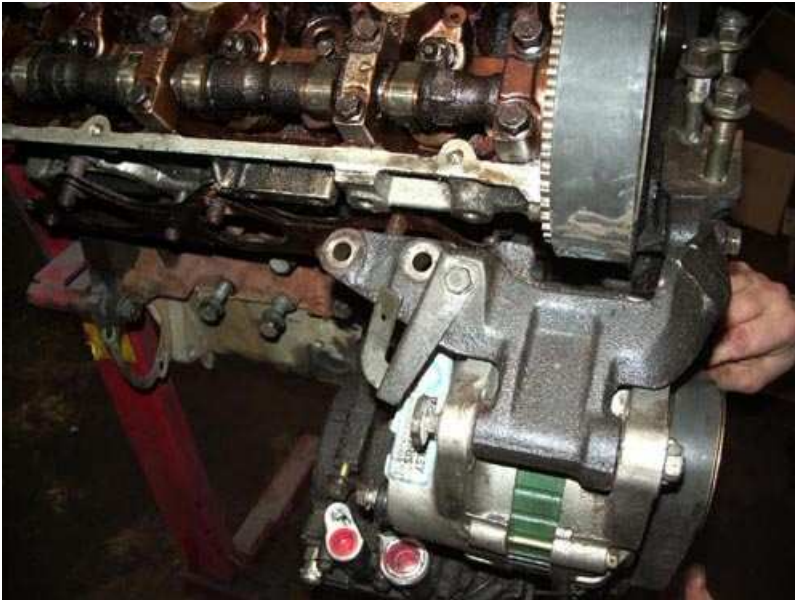
A 6g72 P/S pump bracket and idler pulley is too close to timing belt idler pulley
