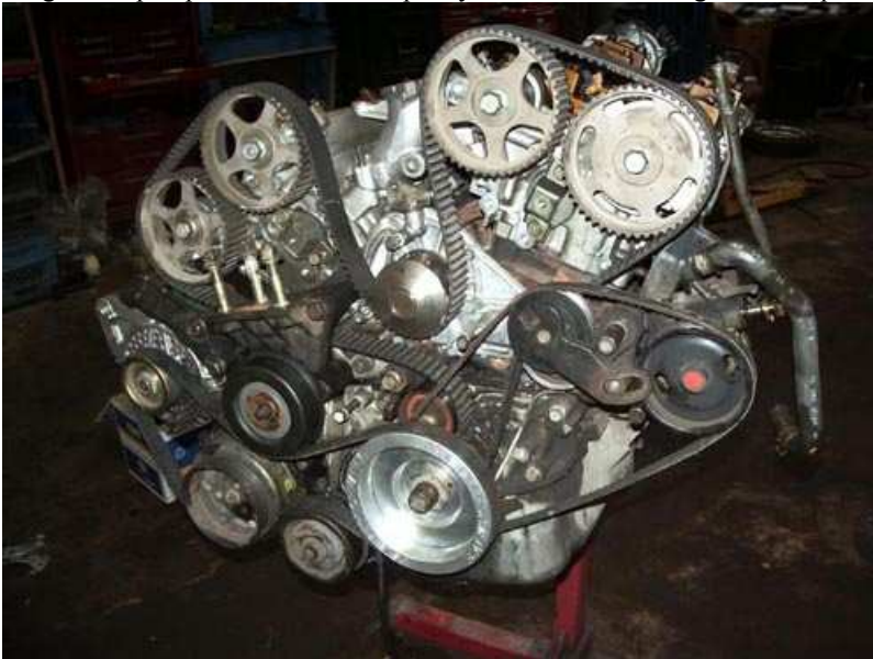
A 6g72 P/S pump bracket and idler pulley is too close to timing belt idler pulley
