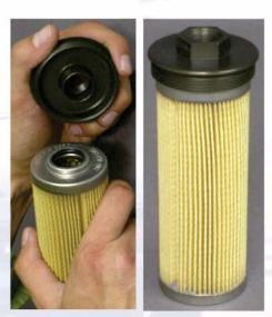
Stainless steel end cap has o-ring on outlet end
