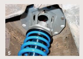
5) To install the shock and bearing housing into mounting plate, slide the entire assembly from below into the guides on the backside of the mounting plate as shown in diagram.
