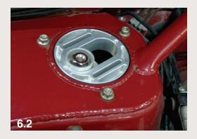
7) Once desired camber is achieved, place the locking plate (C) over top of the bearing housing (B). The locking plate can go in any direction, choose the orientation that allows a clear passage to secure the locking bolt into the mounting plate as indicated.
