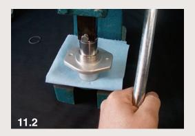
12) Using a pair of snap ring pliers, install the circlip into the groove above the bearing. If no groove is visible, the bearing must be pressed further into the housing. Repeat step #11. Once in place, tap a 21mm socket on the circlip to assure proper engagement into the groove as in **DIAGRAM** # 12.2.
