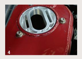
4) Install mounting plate (A) assembly into car as normal and torque nuts to 14.5 ft/lbs. <u>DIAGRAM # 4</u> shows the RH mount in the Camber / Caster position. Mount is now ready to accept the strut assembly.
