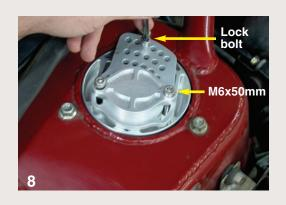
8) Secure the locking plate using the supplied m6 x 20mm lock bolt. The long m6x 50mm bolts are used to lock the name plate (D) onto the bearing housing. Tighten all bolts firmly by hand. Be careful not to over tighten, as you may strip the aluminum threads. See addition comments in **SECTION # C**.
