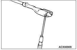
3. Insert a screwdriver through the hole provided on the terminal and raise the contact point. Lightly squeeze the outer edge so the flats are parallel with the bottom.
