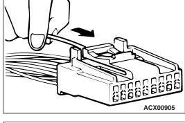
3. Insert the tip of the screwdriver [1.4 mm (0.06 inch) width] into the connector as shown in the figure, gently push the housing lance down with the tip, and pull out the terminal.
