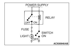
3. By using a relay, a heavy current can be turned on and off by a switch using much less current. For example, in the circuit shown here, when the switch is turned on (closed), current flows to the coil of the relay. Then, its contact is turned on (closed) and the light comes on. The current flowing through the switch is much less than that for the light.
