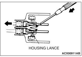
2. Insert the tip of a screwdriver [0.8 mm (0.03 inch) width] into the connector as shown in the figure, push it lightly to raise the housing lance, and pull out the terminal.
