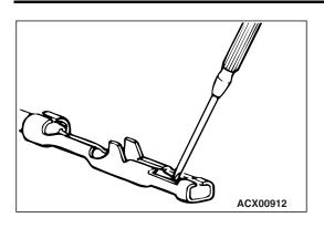
3. Press the contact point to the male terminal down by holding a screwdriver [1.4 mm (0.06 inch) width] as shown in the figure. Lightly squeeze the outer edge so the flats are parallel with the bottom.
