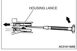
4. Insert a needle through the hole provided on the terminal and raise the contact point. Lightly squeeze the outer edge so the flats are parallel with the bottom.
