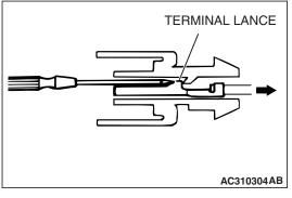
2. Insert the tip of a screwdriver [1.4 mm (0.06 inch) width] into the connector as shown in the figure, press in the terminal lance, and pull out the terminal.
